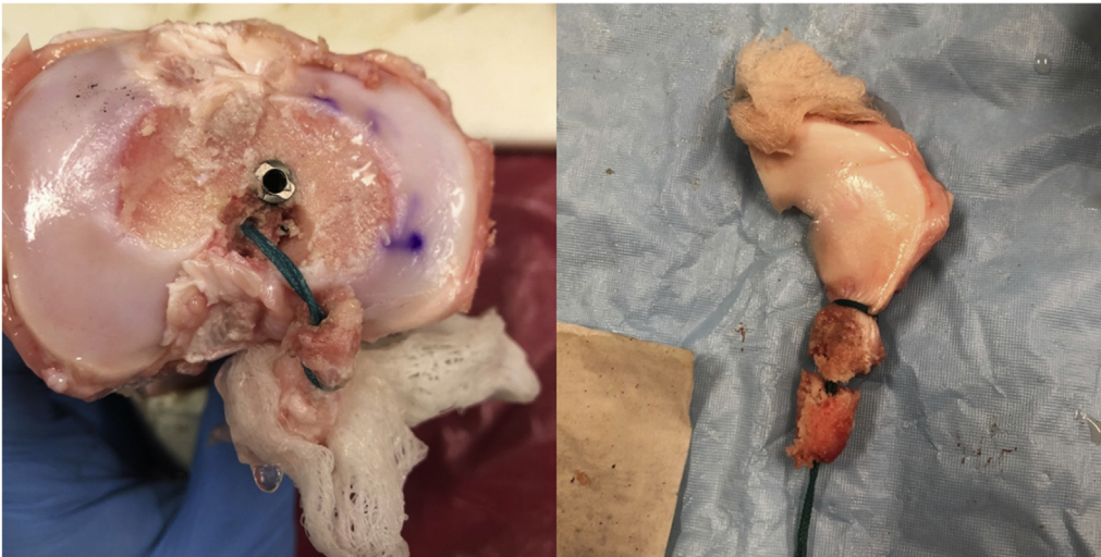
Fig 5. Bone plug breakage as the mode of failure with interference fixation.
