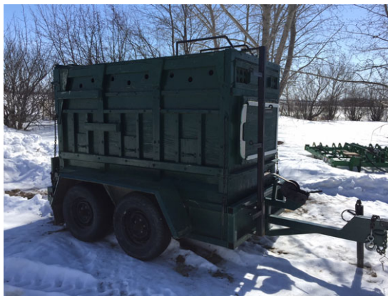
Fig. 3 Side view of the custom built cervid squeeze chute with tilt capability.
