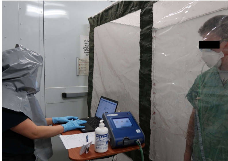
Fig 3. Total inward leakage test being performed on the 3M™ model 9210 N95 FFR. The Sampling probe for the TSI PortaCount 8038 is shown to be connected to the respirator by use of a sampling probe supplied by TSI. The operator is shown to be wearing a loose-fitted PAPR and nitrile gloves as a health and safety precaution from working in close proximity to the test volunteers during the COVID-19 pandemic.
