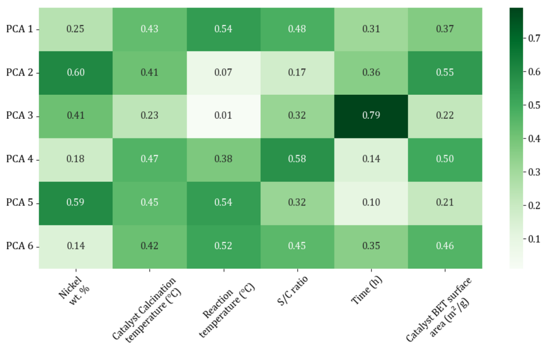
Figure 3. Correlation heatmap of catalyst input features.
