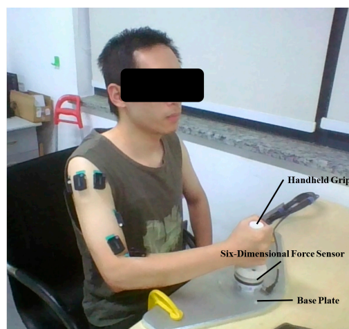
Figure 14. Isometric contraction experiment.
