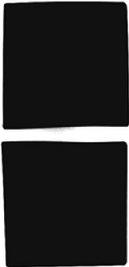
Figure 6 Exposed film demonstrating distinct radiation fields on the skin when the C-arm was rotated between 12° LAO and 12° RAO (16 cm field of view (FOV) on Artis zee, Format group B). The top of the image representing the right side of the anthropomorphic phantom representing a medium patient, and therefore irradiation at the 12° LAO angle. The window/level was adjusted to clearly delineate the two fields (LAO, left anterior oblique; RAO, right anterior oblique).
