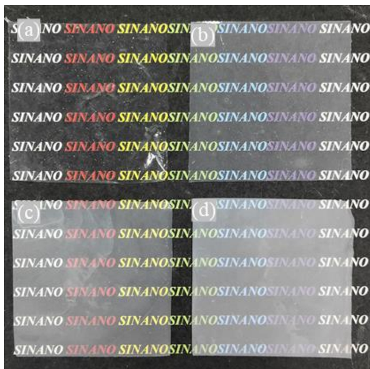
Figure S1. Photo images of the TPU films prepared by solution casting: (a) TPU (SC); (b) AFTPU-10 (SC); (c) AFTPU-15 (SC); (d) AFTPU-25 (SC).
