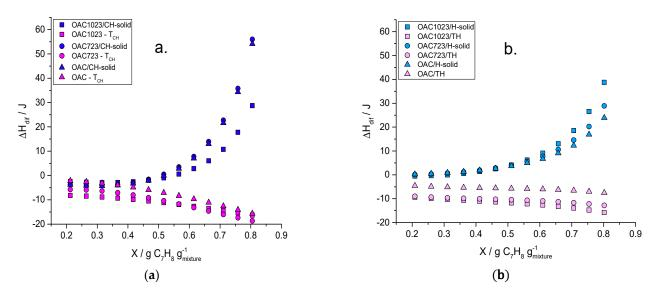
**Figure 7.** Differential enthalpies of toluene and solvent–solid component: cyclohexane–solid (**a**) and hexane–solid (**b**) in function of the mass fraction of  $C_7H_8$ .
