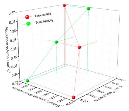
**Figure 2.** Relationship between the micropore volume and the surface area with the total acidity and basicity content of samples.
