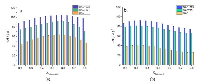
Figure 6. Immersion enthalpies of samples into toluene–cyclohexane (a) and toluene–hexane (b) mixtures.
