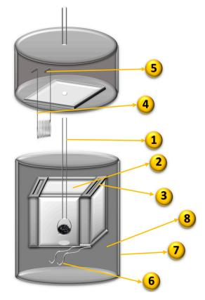
**Figure 9.** Scheme of the heat conduction microcalorimeter: 1. Glass bulb with fragile brittle end; 2. Cell for the liquid of immersion; 3. Sensors; 4. Resistance; 5. Output connection to power source; 6. Output connection to the multimeter; 7. Cover for insulation; 8. Heat dissipator. Adapted and modified from [73], p. 171.
