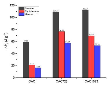
Figure 5. Immersion enthalpies of samples into toluene, cyclohexane and hexane.
