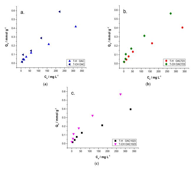
**Figure 3.** Experimental data of liquid-phase isotherms for the adsorption of solutions of toluene in hexane and cyclohexane for OAC (**a**), OAC723 (**b**) y OAC1023 (**c**).
