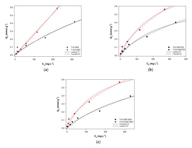
**Figure 4.** Liquid-phase isotherms for the adsorption of solutions of toluene in hexane (T-H) and cyclohexane (T-CH) for OAC (**a**), OAC723 (**b**) y OAC1023 (**c**) adjusted to Freundlich and Langmuir models.
