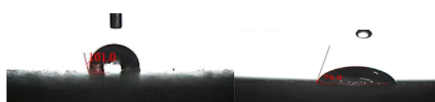
Figure 9. Wetting reversal before and after the action of Bio-Nano30 on the core (oil wet to water wet).
