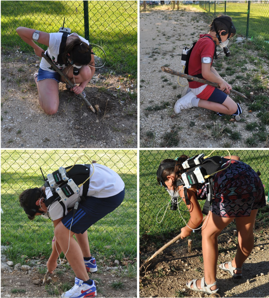
Fig. 1 Volunteers simulating digging tasks with the help of wooden sticks. Energy expenditure was monitored using an Oxycon Mobile JAEGER.® portable device
