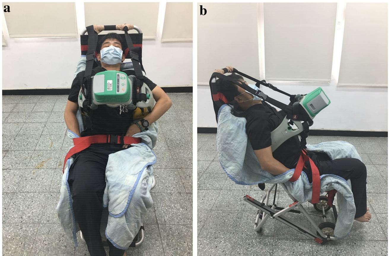
Figure 1. Adaptations of LUCAS-2 mechanical chest compression device enabling its operation in upright position during transportation. (a) Anterior view of simulated patient. (b) Lateral view of simulated patient.
