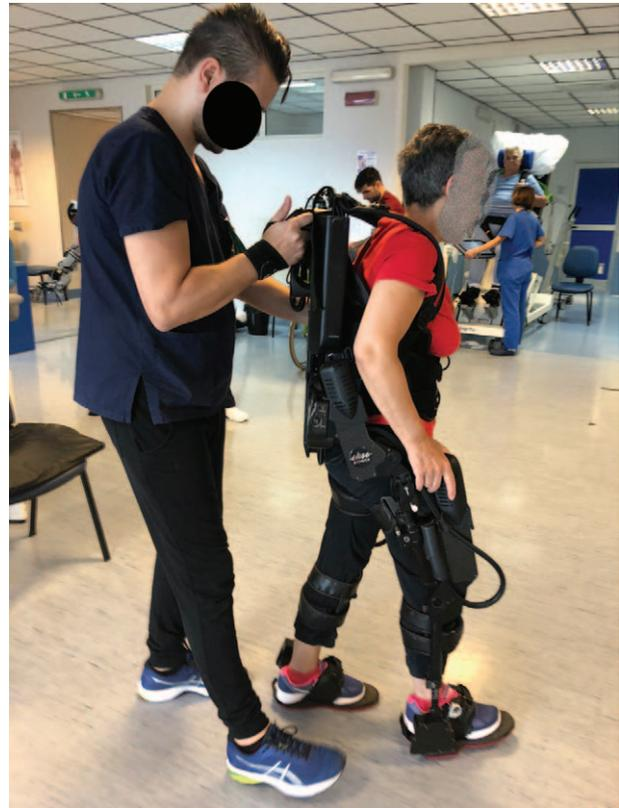
**Figure 1.** shows a typical rehabilitation training with the overground exoskeleton Ekso-GT.
