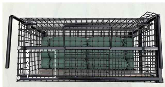
Figure 4. View of front of restraint cage showing left sliding panel (to access hindfoot) open (dashed white line). An identical sliding panel is present on the right side of the cage, to accommodate a badger facing in either direction.
