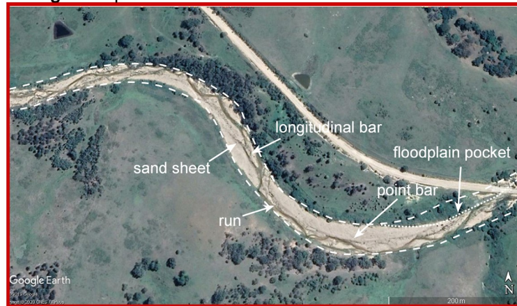
Fig 3. Geomorphic condition principles for a Confined floodplain pockets sand bed River Style in Bega catchment. Uses same examples as in Fig 4. Source of photos; Google Earth and K. Fryirs.
