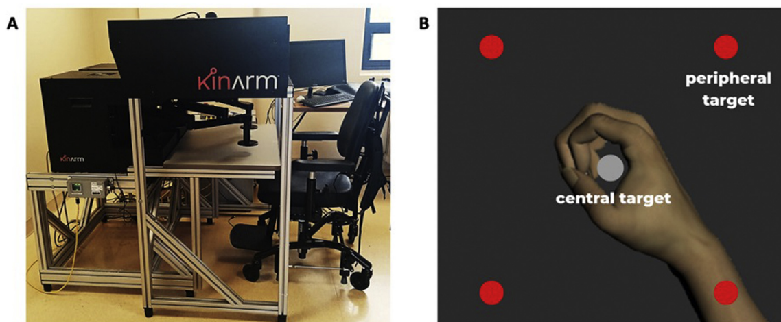
Fig 1 Kinarm End-Point VGR Test. (A) Kinarm End-Point Lab. (B) Screenshot of the VGR test with all peripheral targets illuminated. Note that only 1 peripheral target illuminates during an actual trial.
