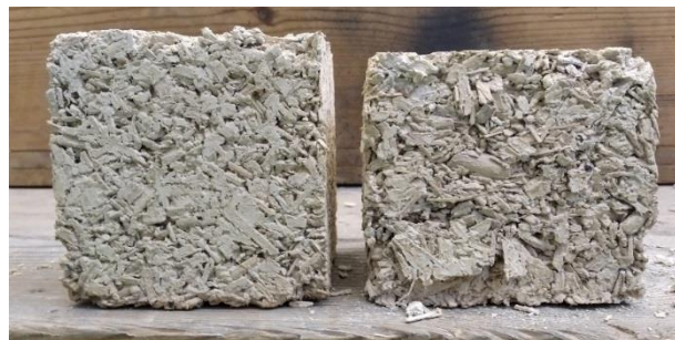
Figure 17. The form of destruction of composite specimen: Original sample (left), damaged sample—15% deformation (right).
