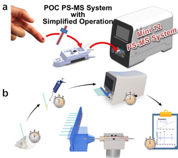
Fig. 13 (a) Mini 12 system that provides a simplified drug-detection operational protocol; (b) detection flow chart. 94 Copyright 2014 American Chemical Society.
