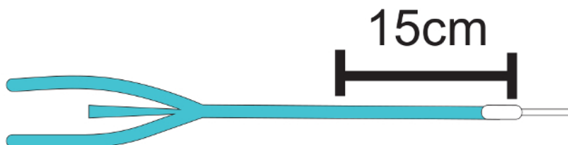
Figure 3. Lubricating the esophageal temperature management device. This schematic illustrates the appropriate procedure for applying water soluble lubrication to the device prior to insertion, as described in step 2.2. Please click here to view a larger version of this figure.
