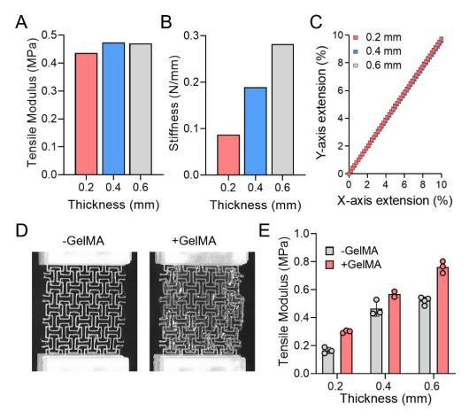
Figure 2. Mechanical properties analysis of orthogonal missing rib substrates according to the different thicknesses and GelMA application. (A) Tensile modulus of missing rib substrates by thickness; (B) Stiffness and (C) X vs. Y extension curves of missing rib substrates by thickness. (D) Tensile test and (E) modulus of missing rib substrates with and without GelMA application. Mean  $\pm$  SD.
