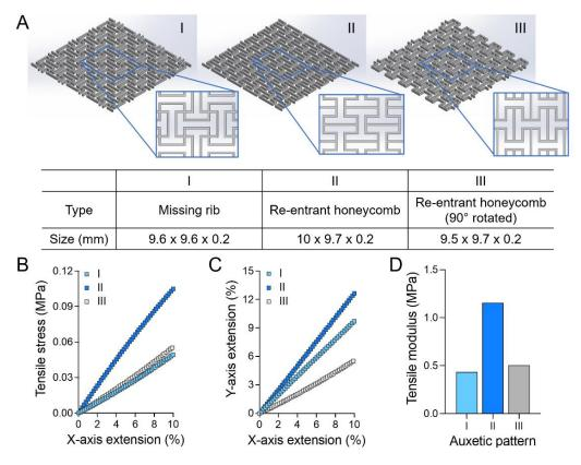
**Figure 1.** Finite element analysis of auxetic patches for the three different patterns. **(A)** Auxetic patch structures of orthogonal missing rib (I),  $0^{\circ}$  (II), and  $90^{\circ}$  (III) rotated re-entrant honeycomb; **(B)** Stress–strain and **(C)** X vs. Y extension curves of auxetic patches; **(D)** Tensile modulus of auxetic patches by patterns.
