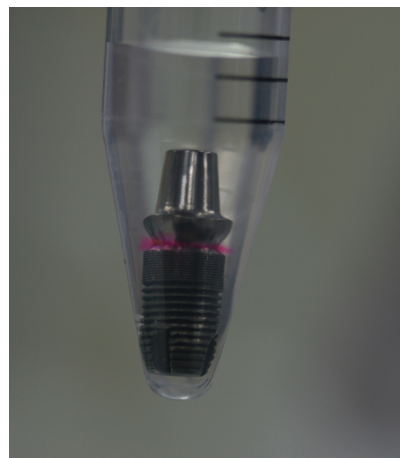
FIGURE 3: The assembly placed in vials filled with 2 mL of distilled water; note the changing of color indicating a leakage of Rhodamine B.
