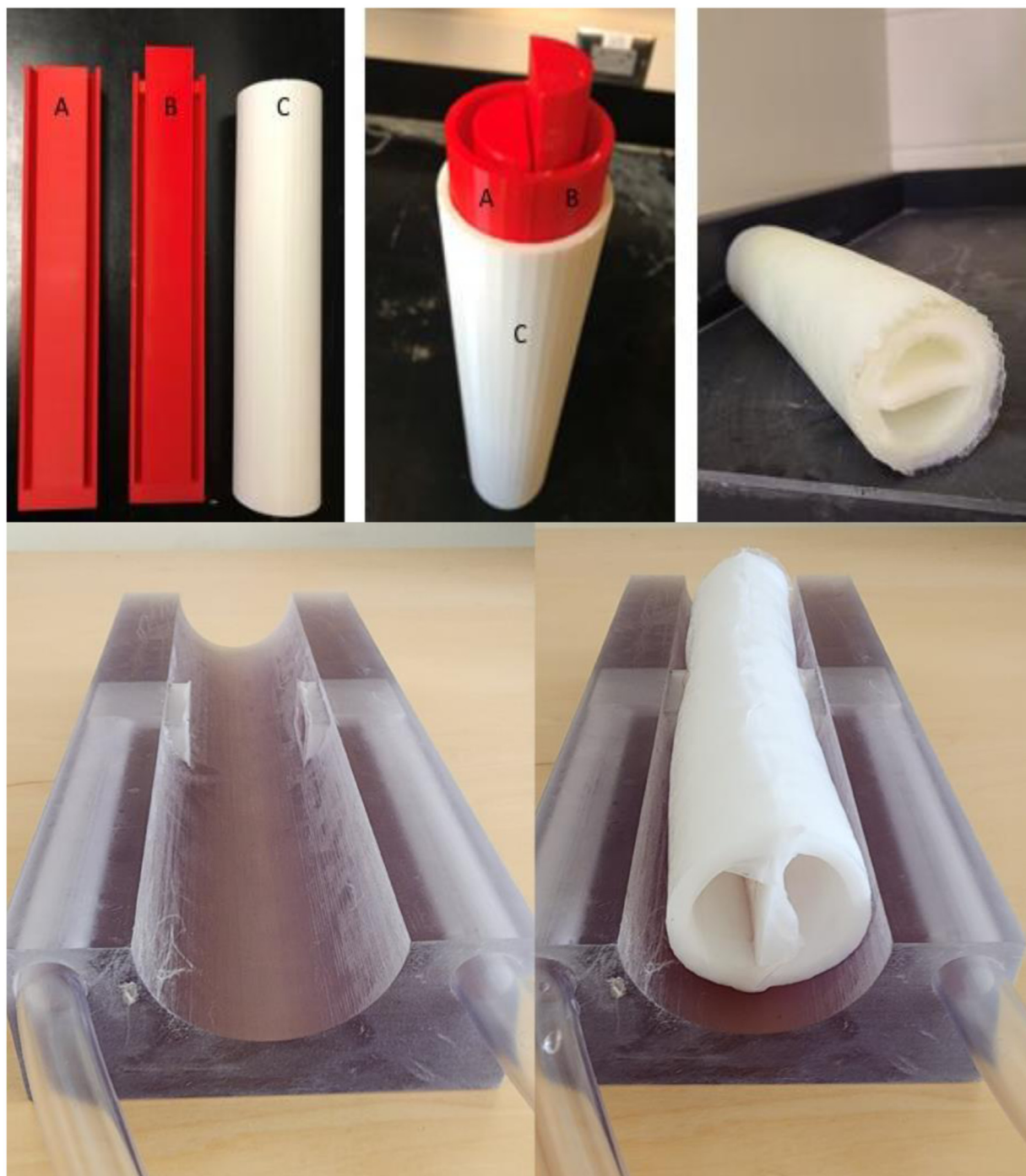
Fig 1. (Top left) Shells A, B, and C, disassembled. (Top middle) Shells A, B, and C, assembled into the mold. (Top right) Cyrogel phantom removed from the mold. (Bottom left) In-house-designed and -built passive driver, with dual diaphragms to deliver vibrations to each side of the phantom separately but simultaneously. (Bottom right) Demonstration of placement of phantom on driver.
