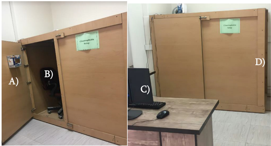
Fig 2. The experiment setup. A) Chamber door that is locked from outside. B) Participant chair for conditions 2-3. C) Data collection setup. D) Moveable wall to allow reduction of chamber space.
