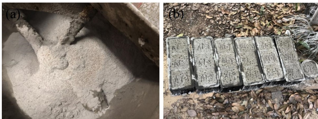
Figure 1. Preparation of the microencapsulated self-healing concrete cube specimens. (a) Adding the microcapsules. (b) Cube test piece before demolding.
