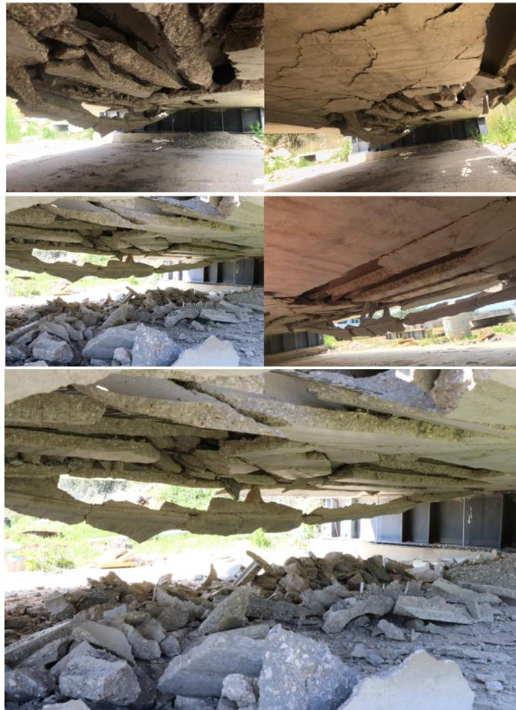
Figure 10. Structural damage from the bottom side after the third impact.
