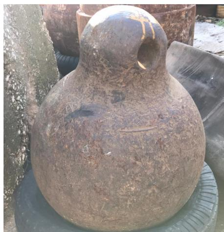
**Figure 4.** The slab Impactor used: 600 kg Steel Ball.
