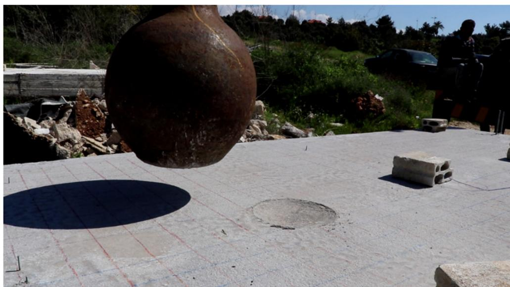
**Figure 7.** Structural damage in the concrete topping from the first impact.
