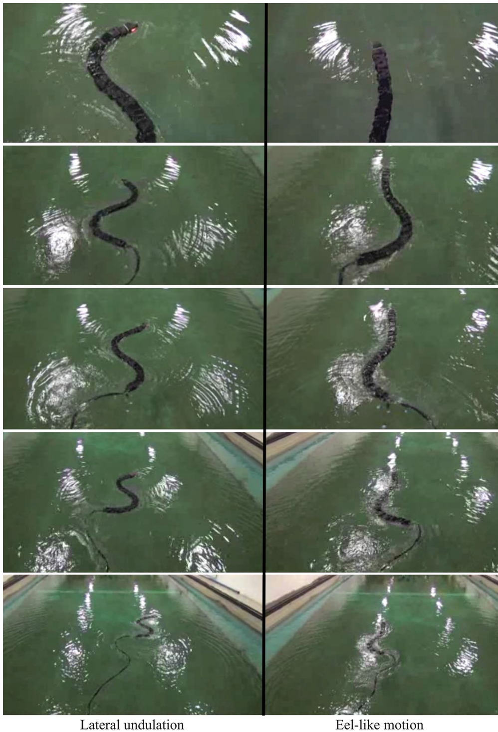
Fig. 11 The motion of the underwater snake robot during lateral undulation and eel-like motion patterns
