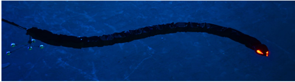
Fig. 3 The underwater snake robot Mamba developed at NTNU to support the research on both ground and underwater snake robot locomotion. Markers are attached to the tail of the robot for position measurements
