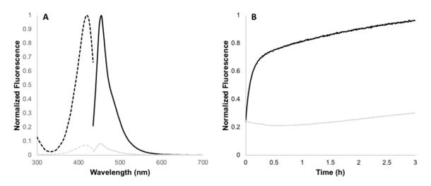
**Figure 1.** (**A**) Excitation (dotted line) and emission (solid line) spectra of **1** before (grey line) and after reacting with MBP-dC10\* (black line). (**B**) Kinetic time course for the fluorogenic reaction between 10  $\mu$ M of **1** with 10  $\mu$ M of MBP-dC10\* (black), relative to the stability of **1** in the absence of MBP-dC10\* (grey). Rate constant  $k_2 = 245 \pm 8 \text{ M}^{-1}\text{s}^{-1}$ .
