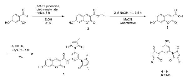
Scheme 2. Synthetic route for the preparation of fluorogen 1.
