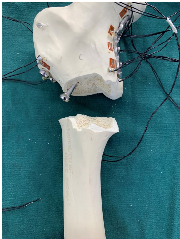
Fig. 4 The sample fractured during the loading process. The fracture site is near the 15 and 16 measuring points, which represents the place where the stress is concentrated
