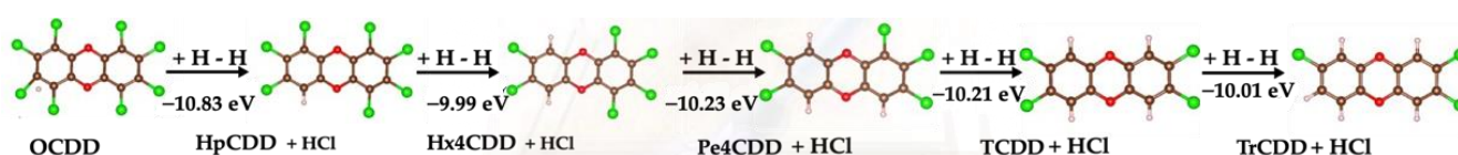
Figure 7. Full consecutive dehydrogenation of the set of PCDDs, from the octachlorodibenzodioxin molecule to trichlorodibenzodioxin. The brown spheres represent C atoms, the green spheres represent Cl atoms, the red spheres represent O atoms and white spheres are H atoms.
