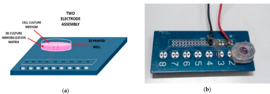
Figure 2. 3D-printed PETG well for cell culture monitoring. (a) Cross section of the cell chamber with the 3D immobilization matrix. (b) Photograph of the well and the electrodes interface. Reproduced from Paivana et al. [29].
