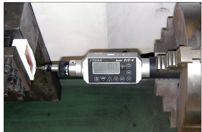
Figure 1: Torque testing unit (milling machine, torque tester, custom-made screw driver, mini-screw and polycarbonate mounted plate)
