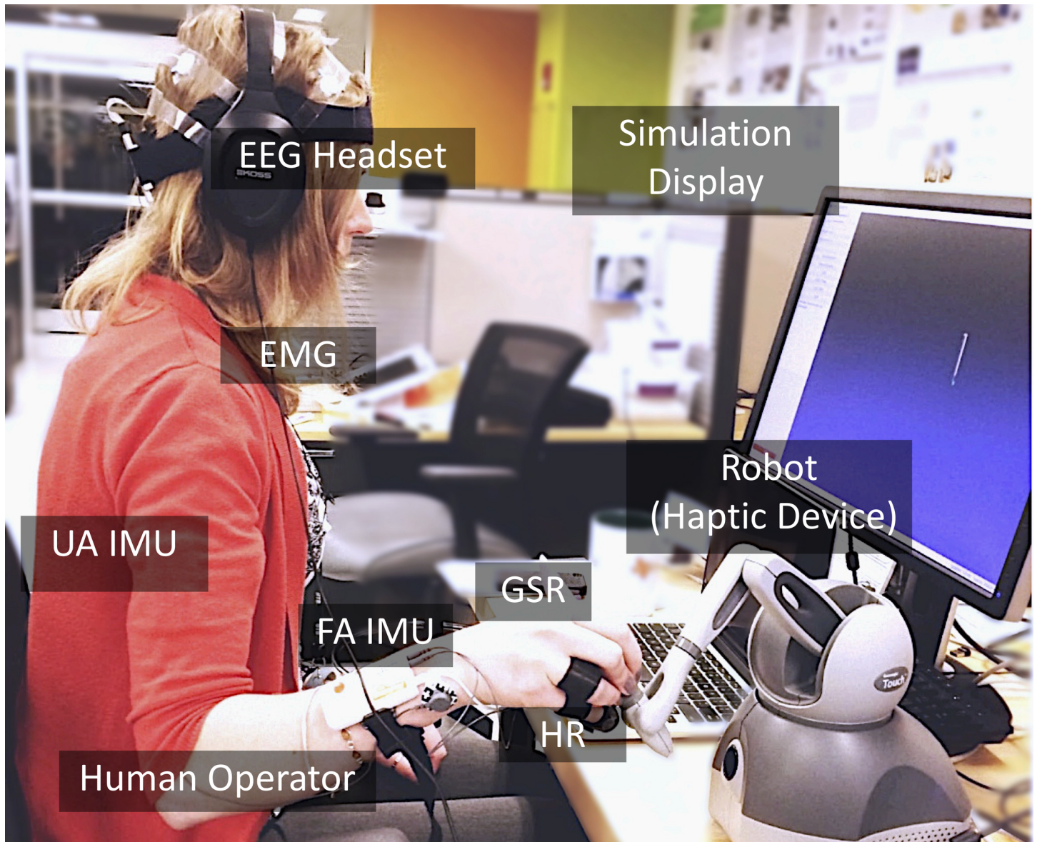
Fig 2. Instrumentation for experiments. Subjects interacted with the virtual task by controlling a robotic interface (i.e., haptic device). Physiological response (e.g., EEG, GSR, EMG) and user kinematic movements were recorded from wireless inertial measurement units (IMUs) on the upper and forearm, as well as encoder readings from the haptic device.
