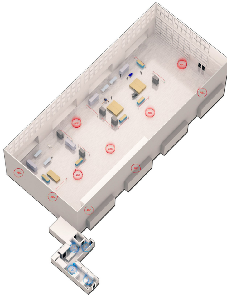
Fig 1. 3D-rendered-model. of sampled controlled cleanroom (CCR) and its uncontrolled adjoining facility (UAF). Triplicate of ten different locations in CCR are indicated by A, B and C (red circles). Samples from four individual locations in UAF are numbered 1 to 4 (blue circles).
