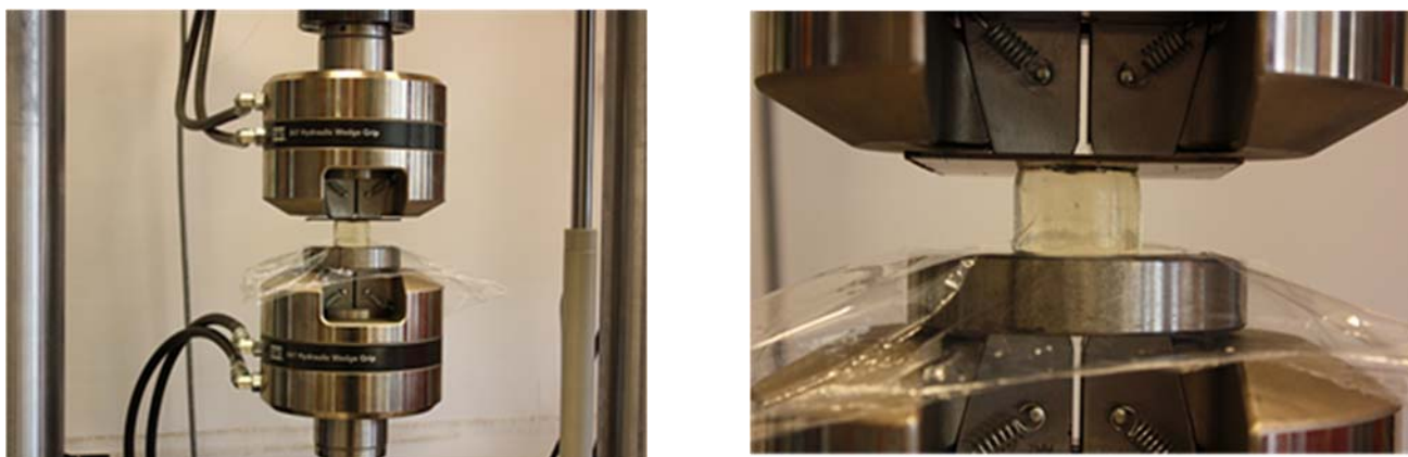
Figure 12. MTS Bionix mechanical testing system equipped with a 1-kN load cell.
