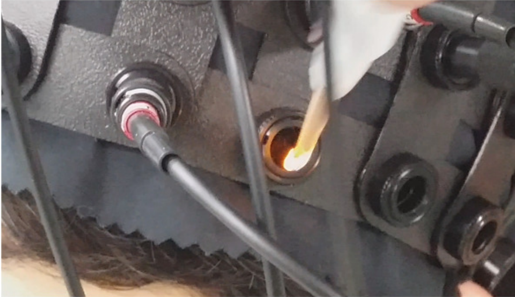
Figure 4: Optimization of optode signals. Hair was moved from each channel using an illuminated plastic tool to displace hair from the channel center to assure optimal signal quality. Please click here to view a larger version of this figure.
