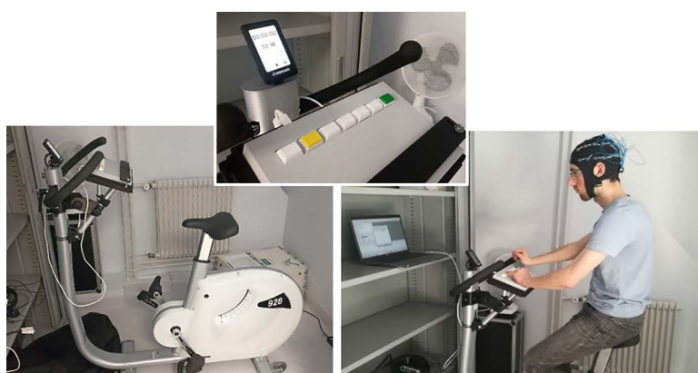
Fig 2. Material used in the study. Left: cycloergometer (Monark 928); middle: response pad; right: EEG cap (Emotiv Epoc Flex).
