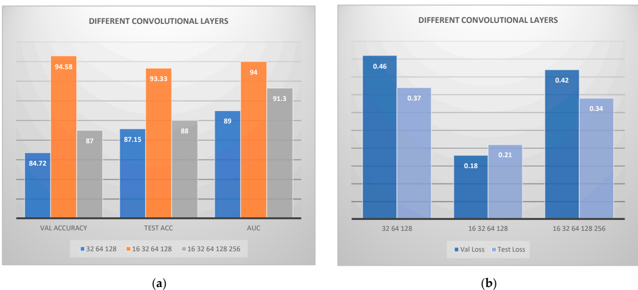
Figure 5. Convolutional neural network architecture for CAD classification problem comparing various convolutional layers: (a) accuracies; (b) losses. VAL is the validation accuracy and ACC is the accuracy.
