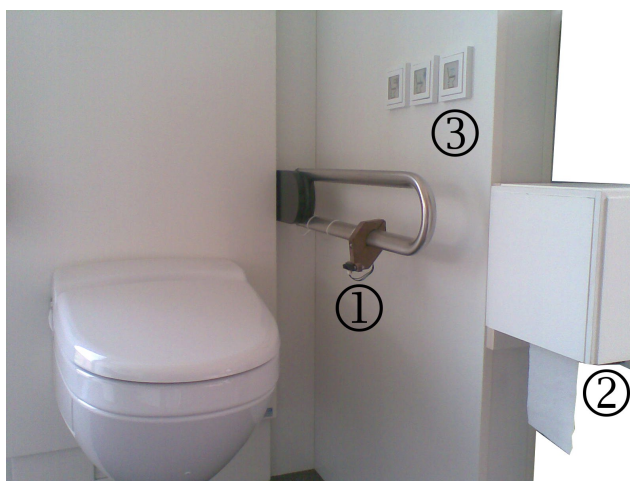
Figure 8. Toilet environment with three sensors: (1) toilet presence; (2) toilet paper use and (3) toilet flush.
