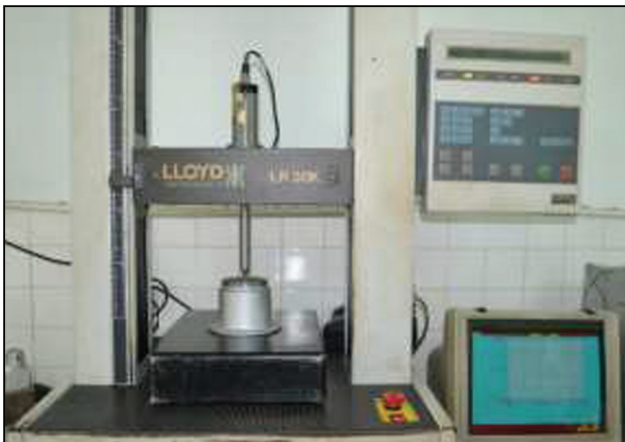
Figure 2: Push-out test apparatus
