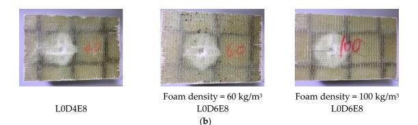
Figure 6. Impact damage with different foam densities.
