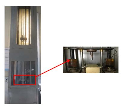
Figure 3. The drop tower apparatus.
