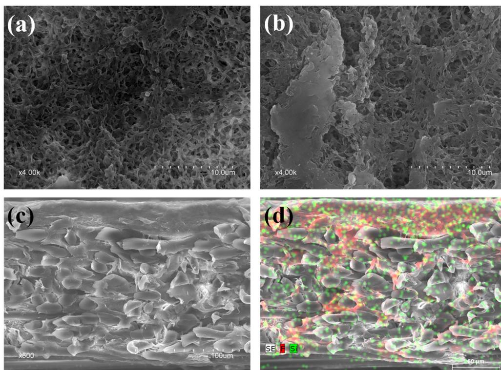
**Figure 6.** FESEM images of (a) non-modified PVDF (nmPVDF) surface, (b) modified PVDF (mPVDF<sub>max</sub>) surface, (c) modified PVDF (mPVDF<sub>max</sub>) cross-section, and (d) EDX mapping of modified PVDF (mPVDF<sub>max</sub>) cross-section (red dots for F and green dots for Si).
