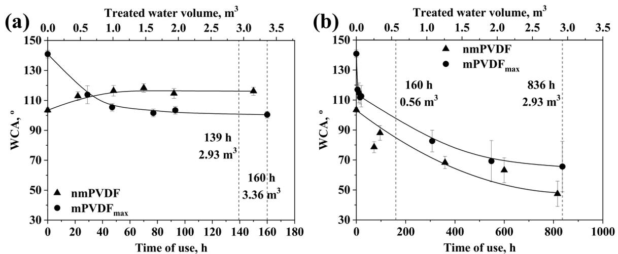
**Figure 7.** Water contact angle versus time of use (bottom axis) and volume of treated water (top axis) for non-modified PVDF (nmPVDF) and PVDF modified under optimal conditions (mPVDF<sub>max</sub>) with (a) deionised water at a liquid flow rate of 21 L h<sup>-1</sup> and (b) anaerobic reactor effluent at a liquid flow rate of 3.5 L h<sup>-1</sup>. Data on nmPVDF with deionised water from [8]. The error bars denote the standard deviation.
