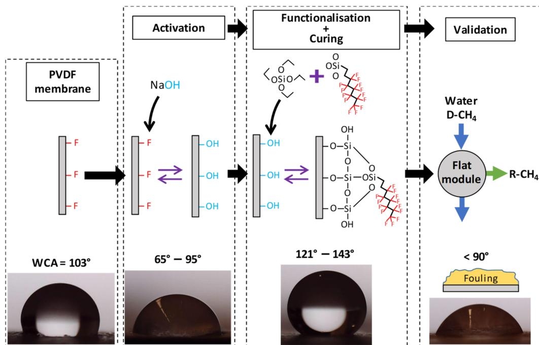
**Figure 1.** Scheme of the modification procedure of poly(vinylidene fluoride) (PVDF) membranes and the validation step. Water contact angle (WCA): static water contact angle; D-CH<sub>4</sub>: methane dissolved in liquid streams; R-CH<sub>4</sub>: methane recovered in gaseous form.
