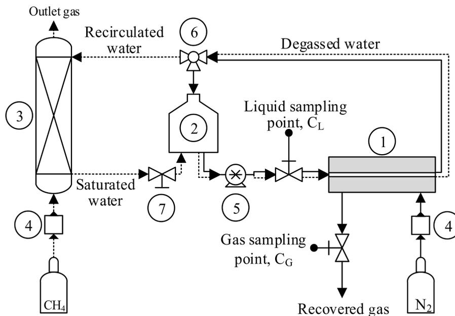
**Figure 2.** Scheme of the experimental system for dissolved methane degassing tests from aqueous streams with a flat-sheet membrane module. (1) membrane module, (2) liquid feed tank, (3) saturation column, (4) mass flow controller, (5) peristaltic pump, (6) 3-way valve, and (7) on/off valve.
