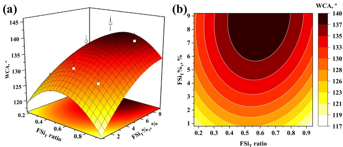
Figure 5. (a) Response surface and (b) contour plot obtained by linear regression from the overall data of the design of the experiments with a  $NaOH$  concentration of 5%. Experimental values are depicted as open symbols in the response surface plot and the error bars denote the standard deviation.
