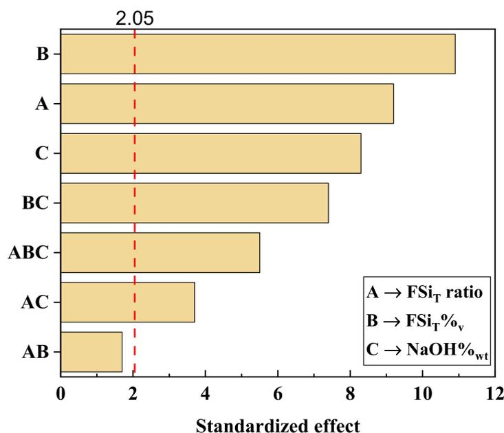
**Figure 3.** Pareto diagram of the standardised effects of the factors analysed in the  $3^3$  complete factorial design. The dashed red line represents the critical standardised effect for a significance level of 0.05.
