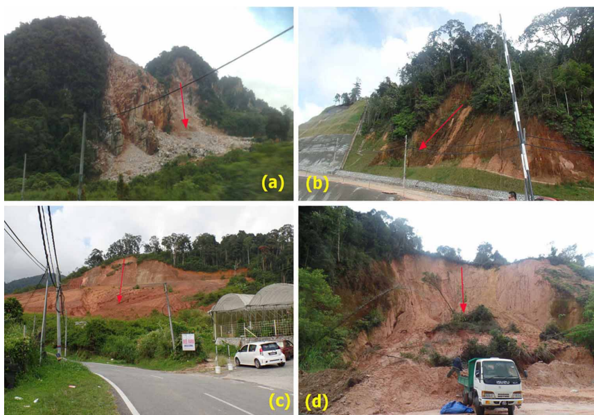
Figure 2 | Field photographs of recently occurred landslides and types of landslides that were taken from field surveys by first author (H. SH); (a) a shallow translational rockslide, (b) a shallow translational debris slide at the road side, (c) and (d) deep-seated rockslides. Arrow depicts the movement direction.
