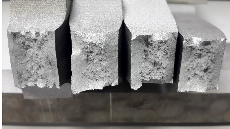
Fig 22. Notched specimens (notch radius 10 mm, 40 mm, and 90 mm from left to right) and smooth specimen after fracture tested at a quasi-static strain rate.
