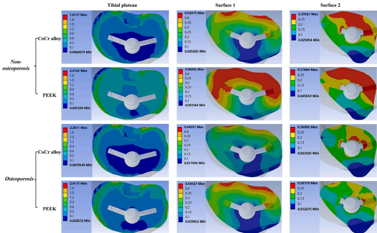
Fig. 2. Nephogram of equivalent stress distribution of tibial plateau and proximal tibia in each model. The blue areas represent stresses of less than 0.1 MPa.
