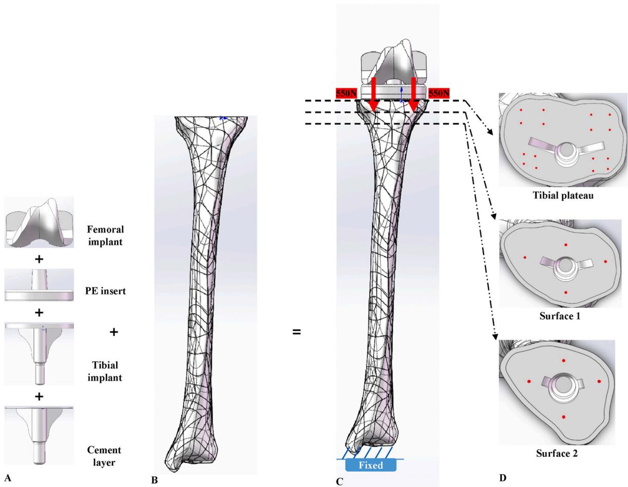
**Fig. 1.** The finite element model including tibial component and 3D model of lower limb. A. Tibial component; B. The assembled model; C. Stress of 550 N was applied to the medial and lateral tibial plateau respectively, and the distal tibia was fixed; D. The stress measuring points on tibial plateau and proximal tibia.
