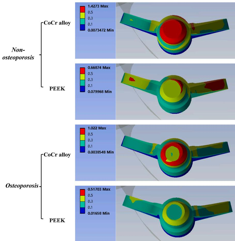
Fig. 3. Nephogram of equivalent stress distribution of distal cancellous bone of tibial implant in each model.
