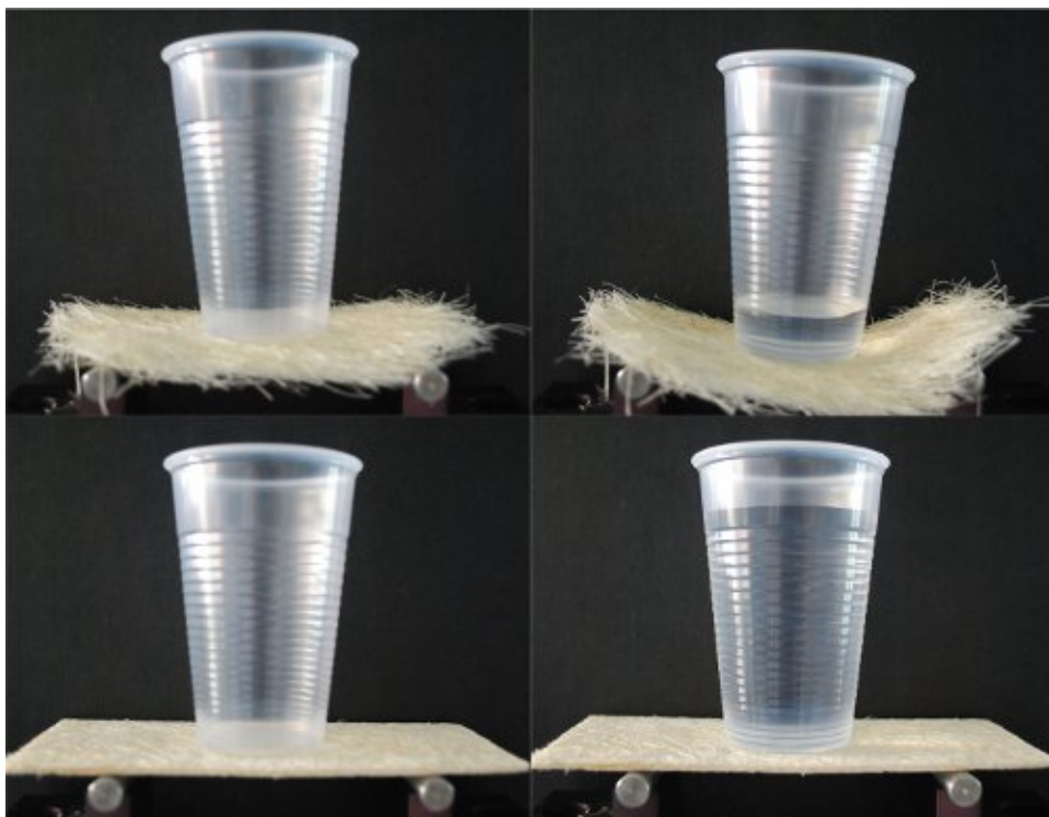
Figure 3. Photographs illustrating the difference in bending stiffness of sisal fiber preforms without (top two images) and with (bottom two images) BC as binder.
