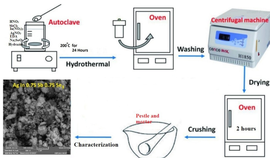
Figure 1. Schematic diagram of the synthesis of \text{AgInSbSe}_3 through hydrothermal technique.
