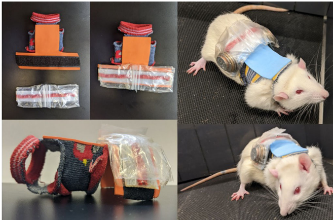
Fig. 1. Rat weighted vest design (left) and a rat wearing a vest containing 15% of its body mass at week 4 of training (right).
