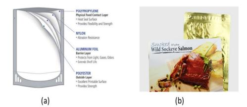
**Figure 4.** (**a**) Retort pouch structural construction (image courtesy: flairpackaging.com), (**b**) commercial retort pouch packaging for smoked salmon.
