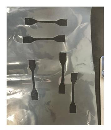
**Figure 4.** Cutting on B (Corn starch, cassava, and eucalyptus) biopolymer film to evaluate the mechanical properties with respect to the lamination direction.
