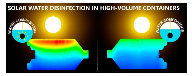
**Figure 6.** Differences in the distribution of radiation inside high-capacity containers for different optically active substances naturally occurring in water. (**Left**) substances with scattering properties. (**Right**) substances with absorption properties [57]. Warn colours (red) mean high values of irradiance, and cold colours (blue) mean low values of irradiance.
