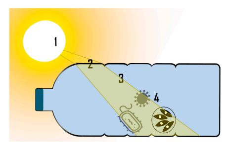
**Figure 5.** The path the radiation travels from the sun to the pathogen in the SODIS process. #1: Radiation source; #2: Crossing through the container; #3: Crossing through the water; #4 Radiation that reaches pathogens.
