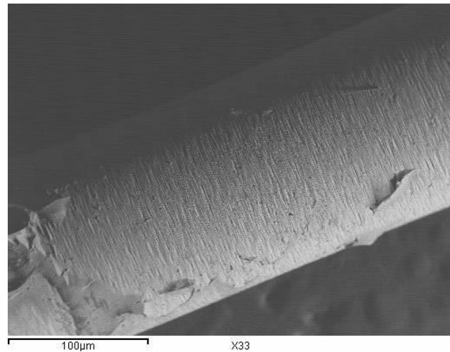
Figure 15 Representative SEM of control group attached to IPS empress core (original magnification 33) demonstrating adhesive/Cohesive type of failure.
